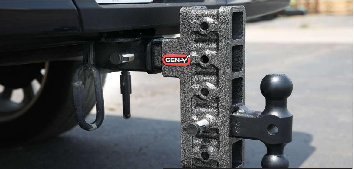
MEGA-DUTY HITCHES CAN BE USED IN THE DROP OR RISE POSITION
