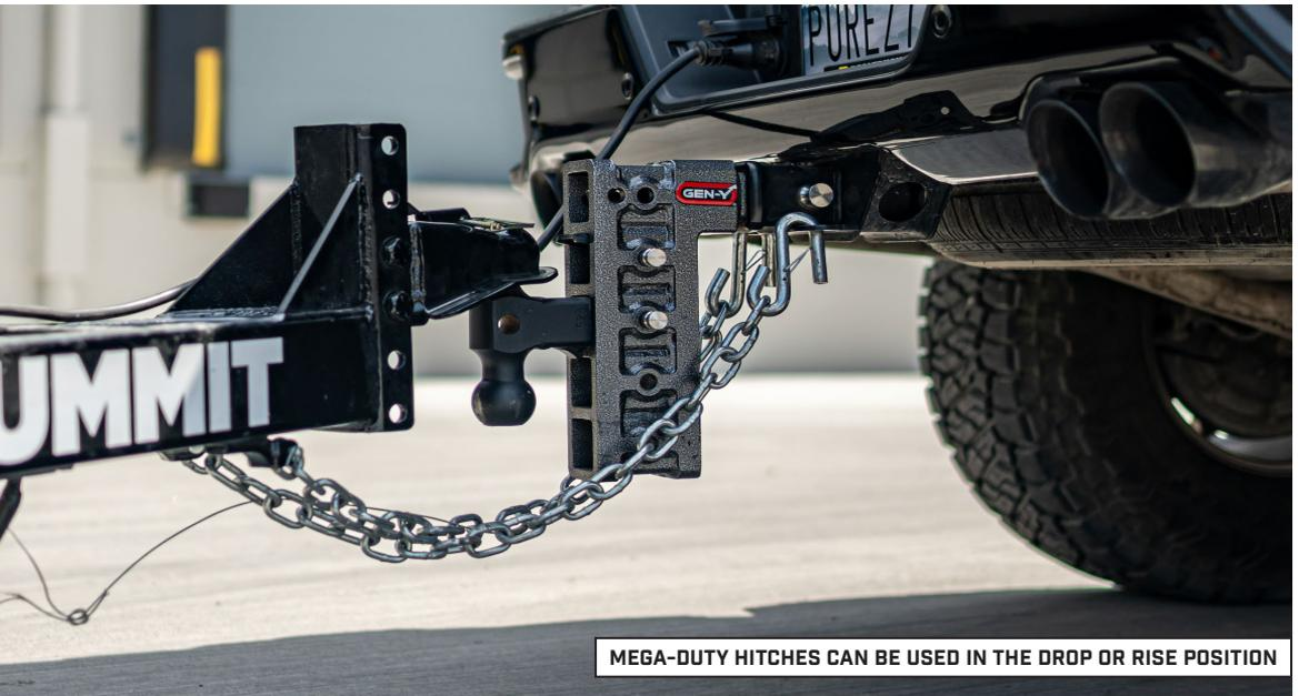
MEGA-DUTY HITCHES CAN BE USED IN THE DROP OR RISE POSITION
