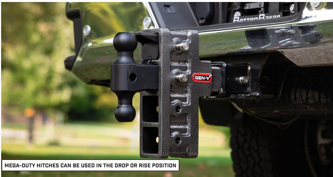
MEGA-DUTY HITCHES CAN BE USED IN THE DROP OR RISE POSITION
