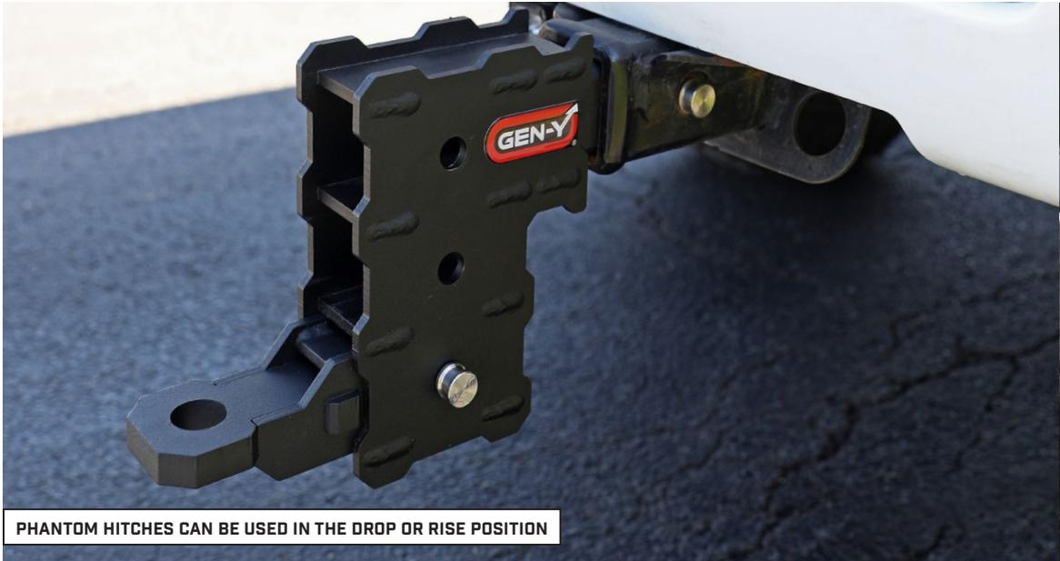
PHANTOM HITCHES CAN BE USED IN THE DROP OR RISE POSITION
