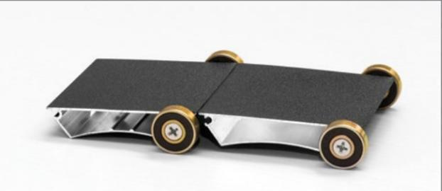
Sealed ball-bearing rollers are mounted onto each section. This allows the retractable cover to open and close easily with one hand, without the need for pull straps, Velcro, snaps or springs. Ball-bearings provide smooth operation, preventing the cover from binding when opening or closing.
