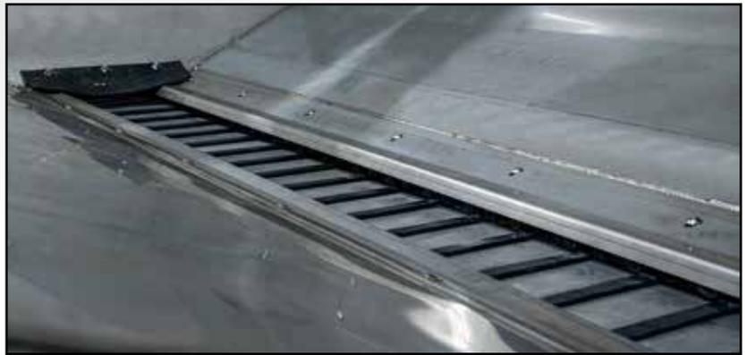
High speed conveyor chain feed, 14-1/2" wide conveyor with 1/4" bars
