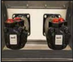
High Torque Auger Motor
