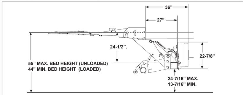
GPTLR-44 & 55 Lift Dimensions and Mounting Requirements
