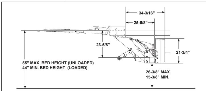
GPTLR-25 & 33 Lift Dimensions and Mounting Requirements
