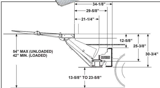
TE-25/TE-30 Lift Dimensions and Mounting Requirements
