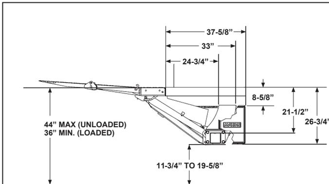
TE-25L/TE-30L Lift Dimensions and Mounting Requirements
