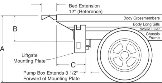
The diagram illustrates the truck mounting requirements with the following labels and dimensions:
